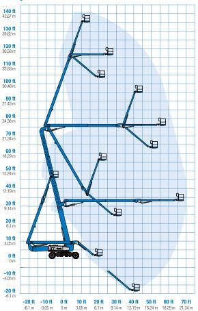
\* The metric equivalent of working height adds 2 m to platform height.
